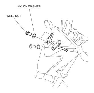
15. Install the meter visor as shown.
