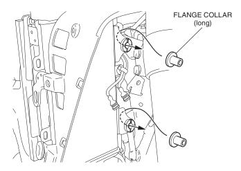
13. Install the horn cover as shown.
