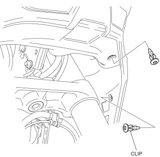
4. Remove the front tank cover as shown. <Left side> CRF1100A/D
